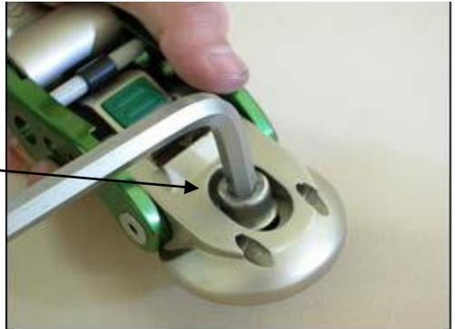
Establish orientation and tighten bolt.
